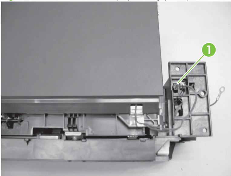
Figure 6-146 Remove the multipurpose tray (4 of 5)
