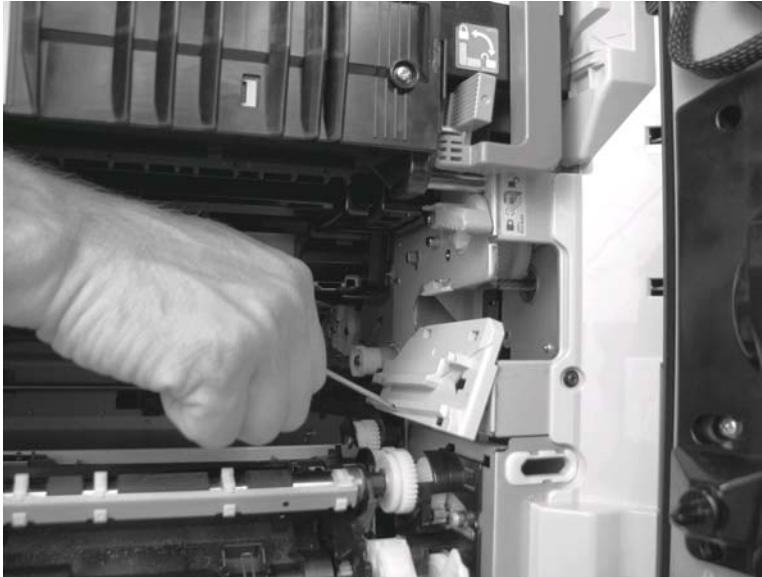
Figure 6-3 Remove the secondary transfer unit (1 of 9)
